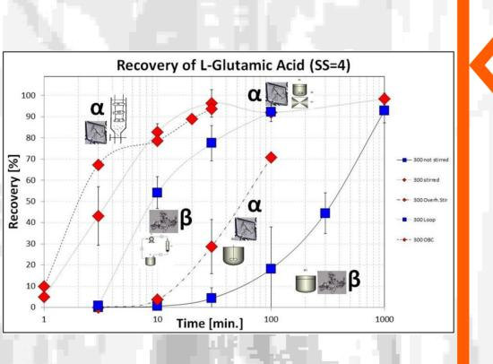
Reactive crystallisation of L-Glutamic acid from Na-L-Glutamate and sulphuric acid aqueous solution, C.F. Roelands (2007)
