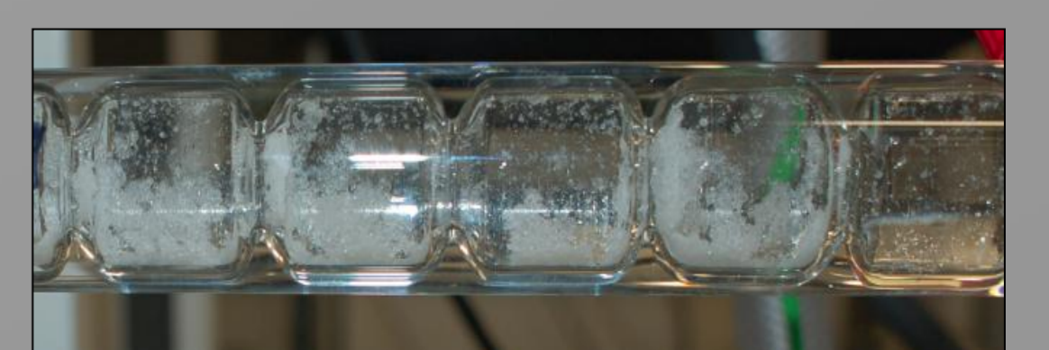
Fig 20 Encrustation on COBC walls
