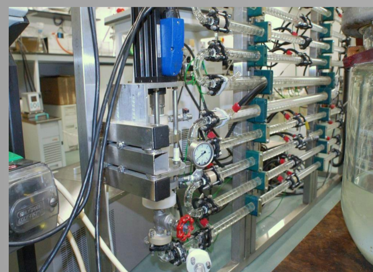
Fig 3 COBC DN15 - working volume of 3.2L
