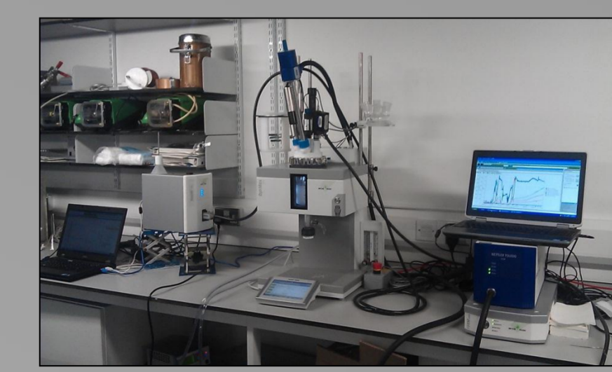
Fig 1 Mettler Toledo Optimax system set up for solubility measurement
