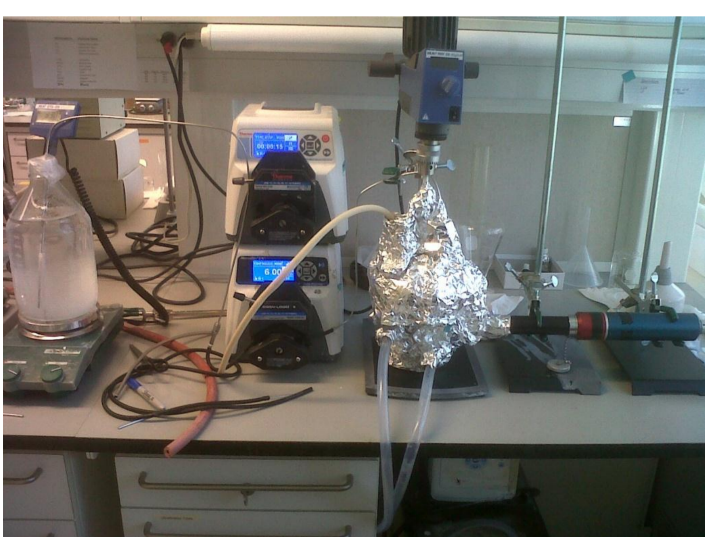
Figure 1 a): Set up of MSMPR b) Phase diagram of alpha and beta LGA showing the liquid phase concentrations at 25°C and 45°C using a 30 min RT
