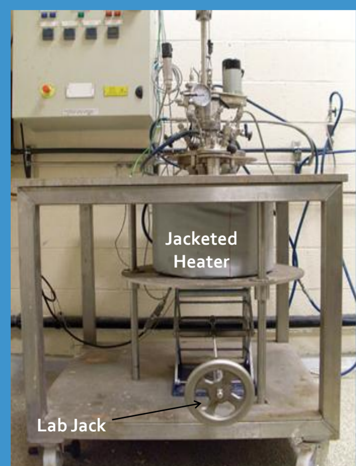
Figure 4. Baskerville pilot autoclave used to digest bauxite ores.
