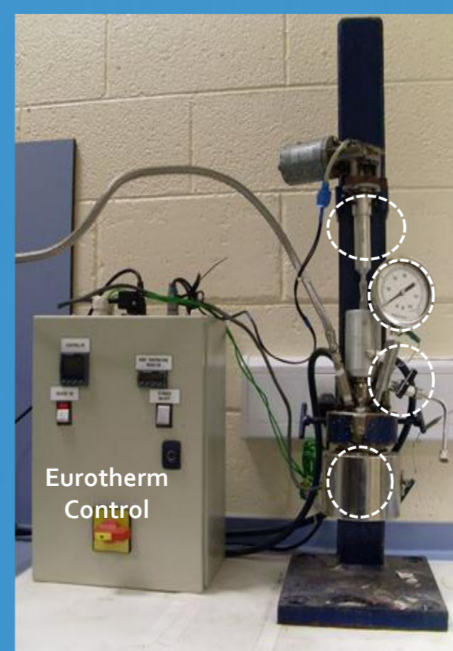
Figure 6. Parr 4560 benchtop autoclave used for digestion.
