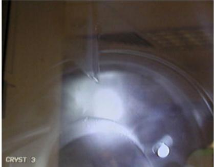
Encrustation was a significant issue during early stages of process development. Operating at low supersaturation minimises the problem. Building a cleaning procedure into the process has made long term operation possible
